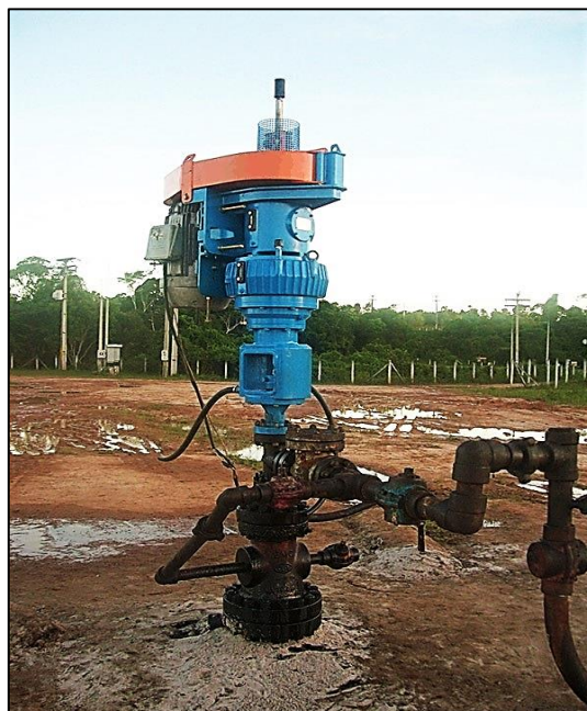
Drive head with hydrodynamic brake retarder in operation
