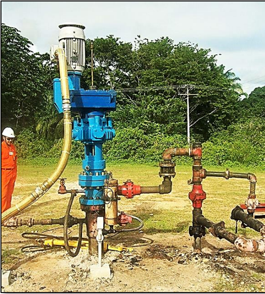
Drive head with hydraulic brake in operation
